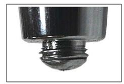
The problem of bubbles coming back up into the color cup or bottle (**picture 1**) occurs when air and paint mix at the point slightly in front of the nozzle. Or, that's the way it's supposed to be. Needless to say, if there is any gap in the paint system, air is going to find it. Also, air in the paint system may show up as a fluttering sound or in the form of pulsing spray.
